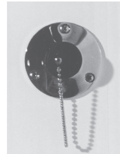
Washdown Hose Connector (Typical)
