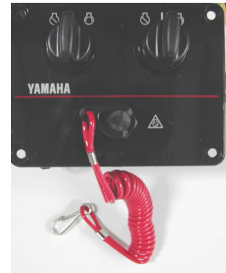
Engine Stop Switch
