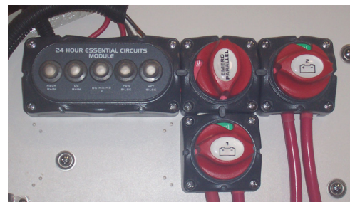
DC Distribution - Twin Engines
