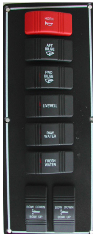
Helm Switch Panel Right
