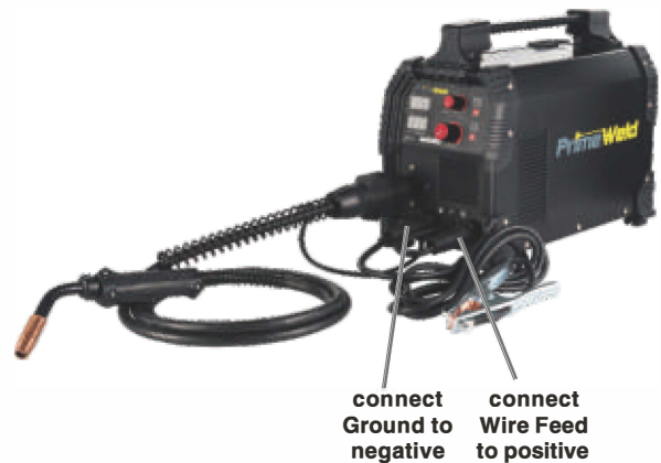
DCEP Solid Core (Gas Shielded) Polarity Setup
