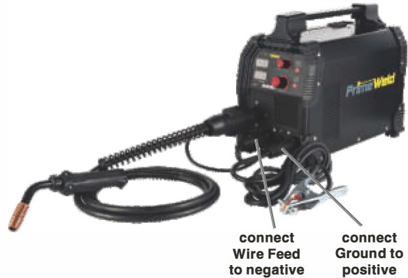
DCEN Flux-Cored (Gasless) Polarity Setup
