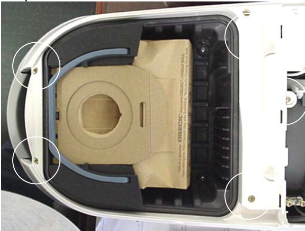
Remove Upper Housing Screws
