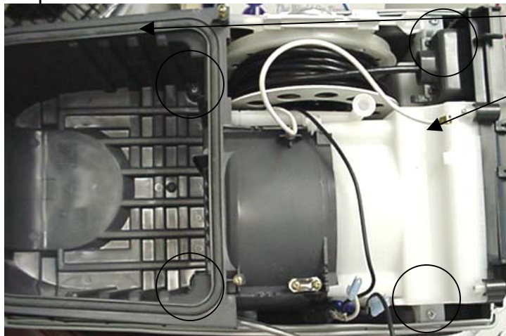
Dust Chamber/Motor Housing/Back Lid Assembly Screw Locations
