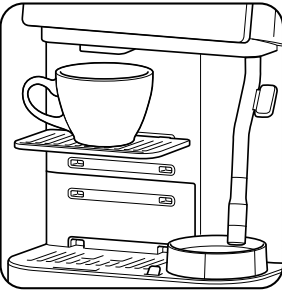
To avoid splatter, use the adjustable cup tray to raise your cup closer to the spouts.
