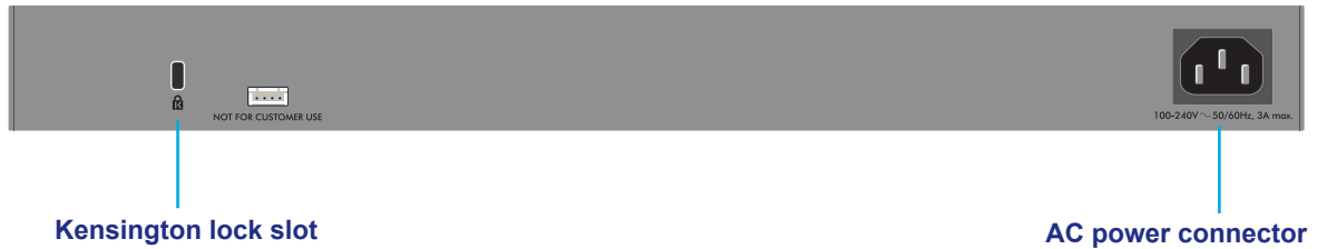
Figure 2. Back panel model XS728T
