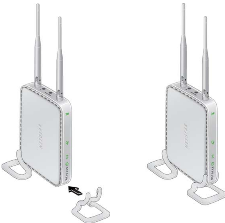
Figure 4. Attach the feet to the access point
