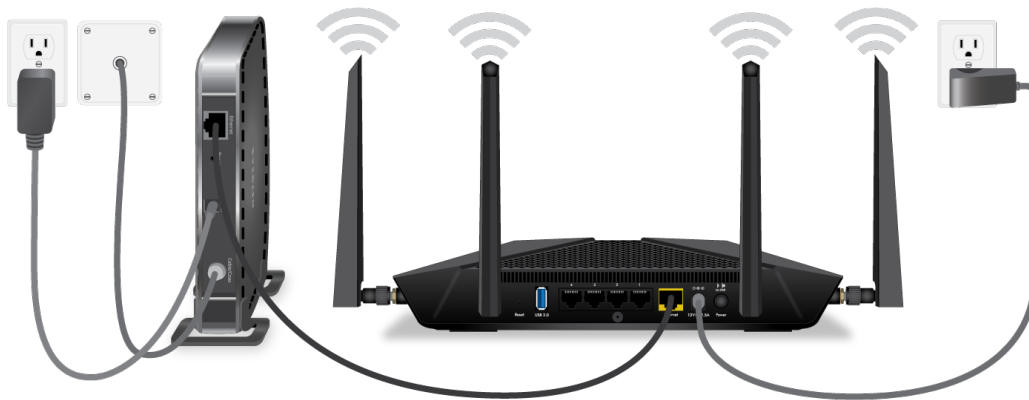
Figure 7. Cable your router
