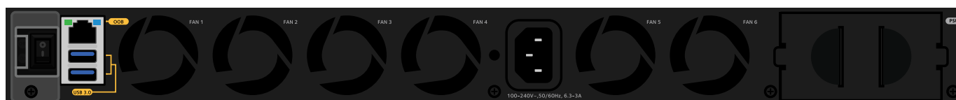
Figure 26. Back panel model M4350-24F4X
