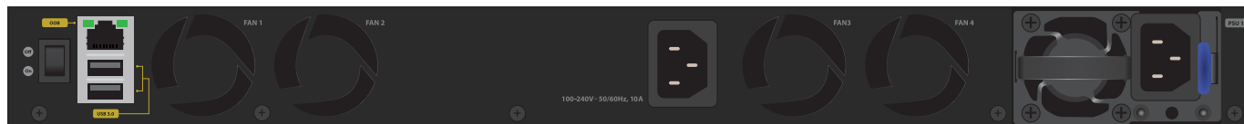
Figure 6. Back panel model M4350-24G4XF
