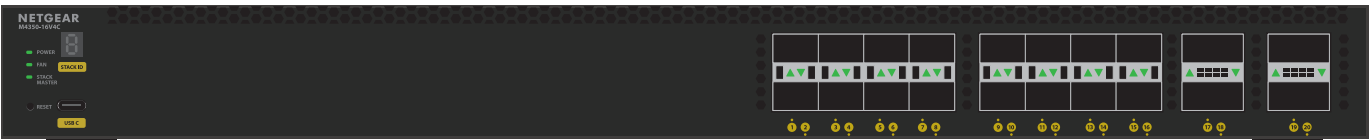
Figure 21. Front panel model M4350-16V4C
