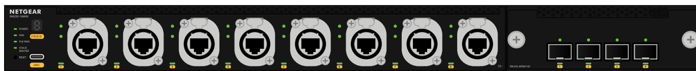
Figure 34. Front panel model M4350-16M4V
