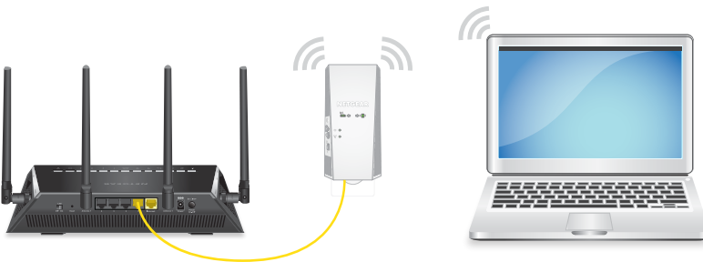
Figure 3. Extender in access point mode
