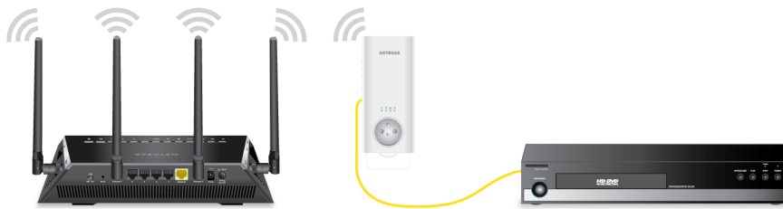
Figure 5. Ethernet-enabled device connected to the extender
