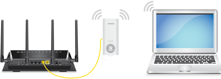
Figure 4. Extender in access point mode
