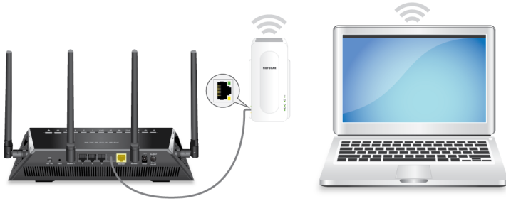
Figure 4. Extender in access point mode
