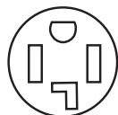
4-wire receptacle (14-30R)
