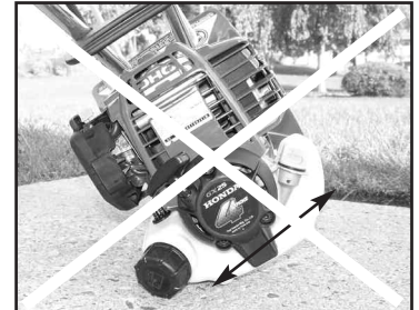
This position does not allow for a proper oil level reading and may cause overfilling.
