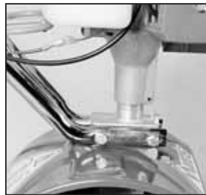
Picture 1 ... Note how the engine doesn't sit all the way down on the transmission.
