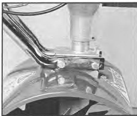
Picture 1 ... Note how the engine doesn't sit all the way down on the transmission.
