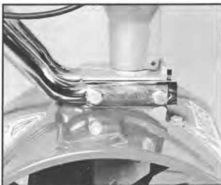
Picture 2 ... Note how the engine sits all the way down on the transmission.
