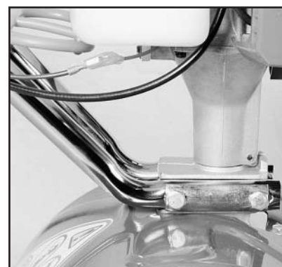
Picture 2 ... Note how the engine sits all the way down on the transmission.
