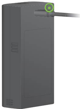
Green - Battery fully charged
