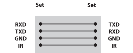
4-Wire Configurations (Standard RS-232C cable)
