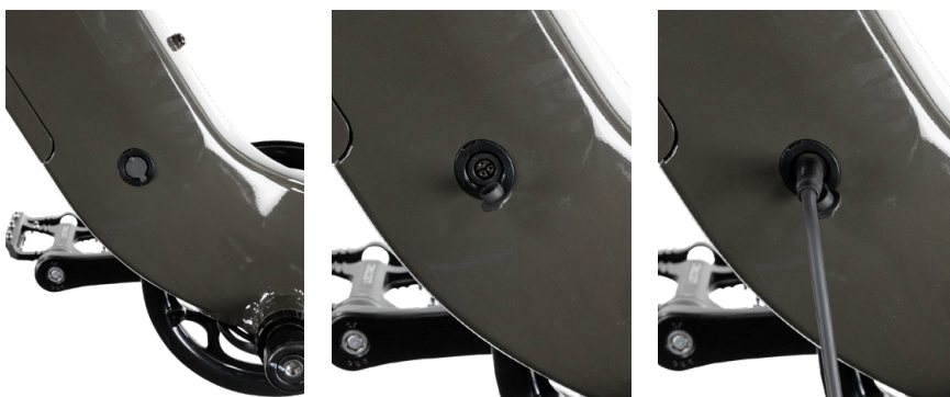
Battery charging in bike frame
