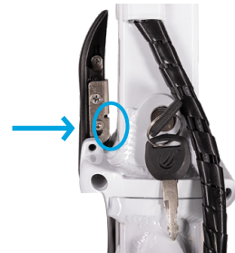
Locking Pin retracted
