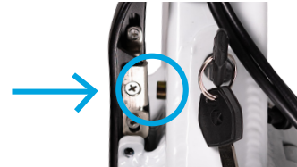
Locking Pin protruding through frame
