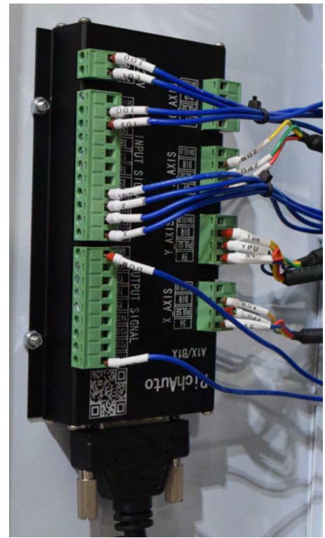
Control board for handheld controller
