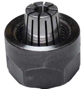
Collet fitted to spindle nut
