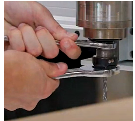
Tightening the spindle nut
