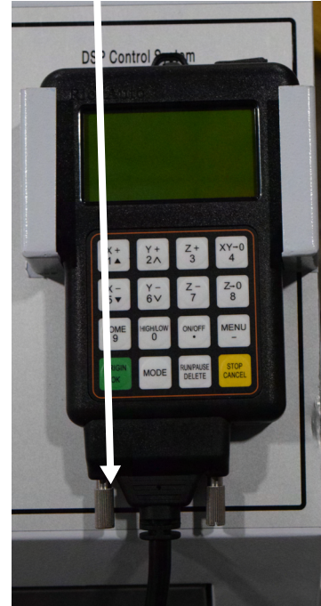
Controller attached to cable
