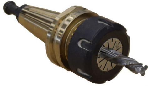
Figure 5-5: Assembled Tool Cone
