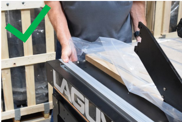
Figure 6-3: Correct Ways to Lift Machine without Forklift
