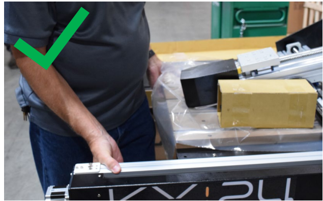
Figure 6-3: Correct Ways to Lift Machine without Forklift
