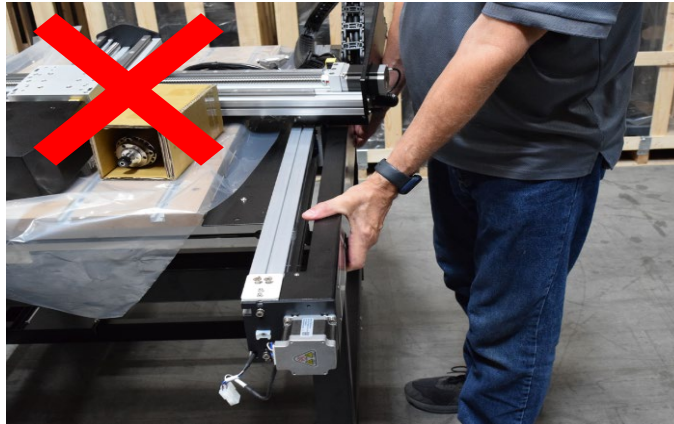
Figure 6-2: Incorrect Way to Lift Machine without Forklift
