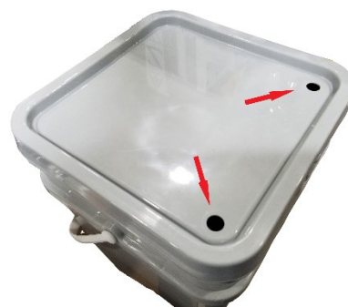
Figure 4-2: Holes for Water Pump Hoses
