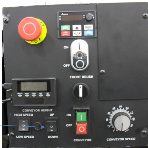
Figure 17: Height Control Adjustment, electronic
