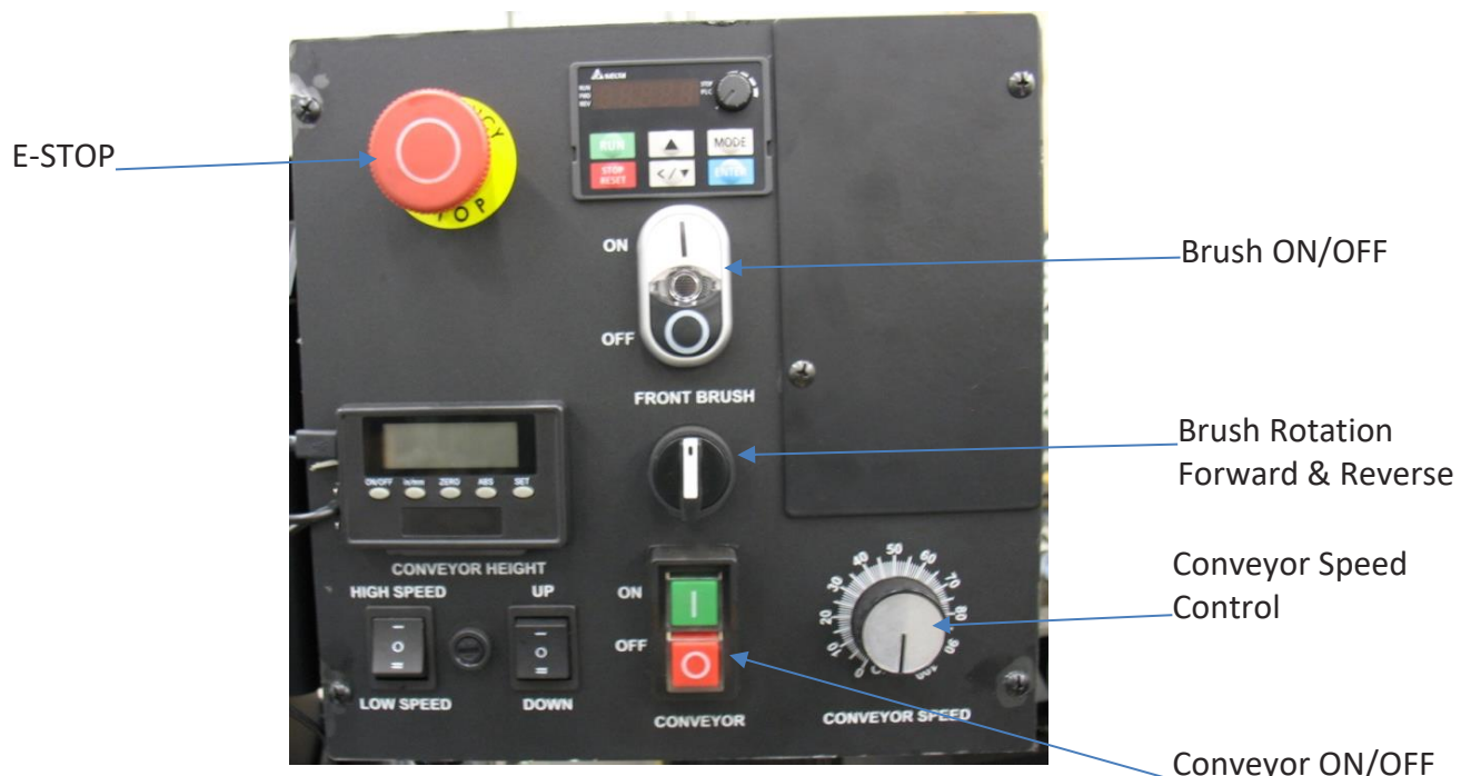
Figure 20: Brush & Conveyor controls
