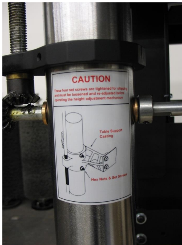
Figure 3: Table Support Set Screws
