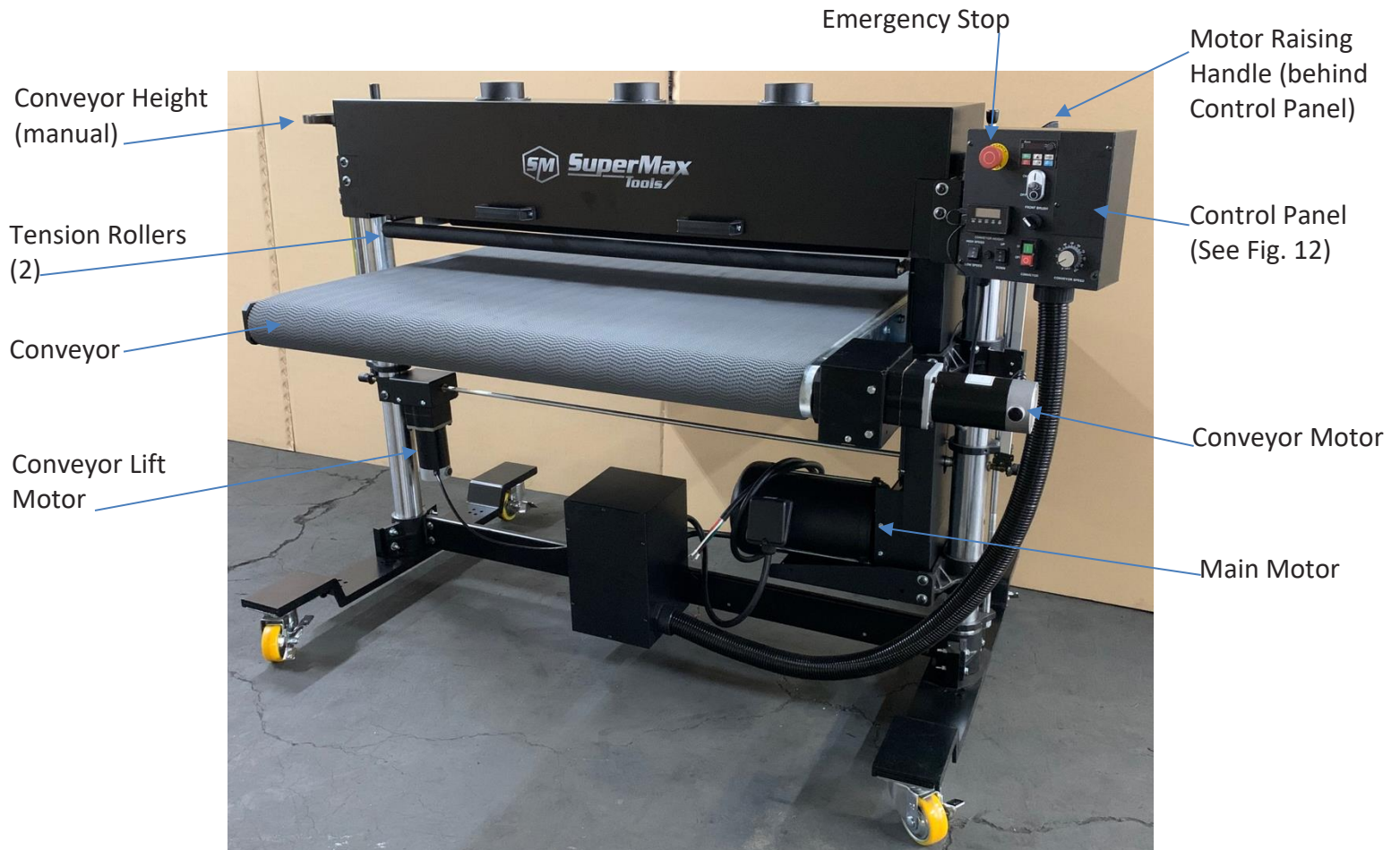
Figure 10: Main Components of SuperBrush 49
