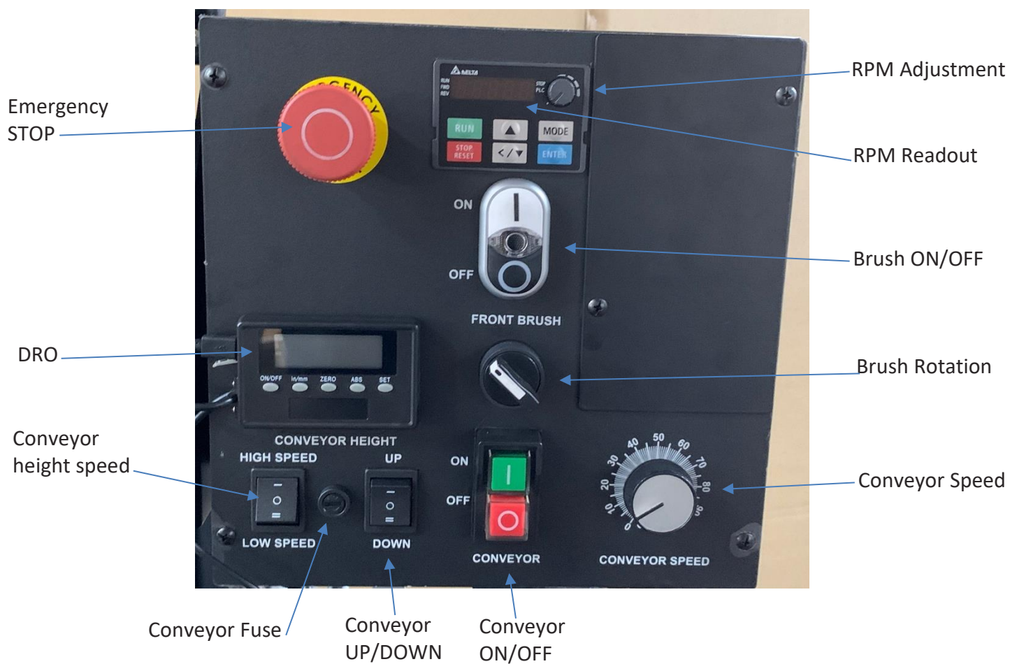
Figure 12: Control Panel Components
