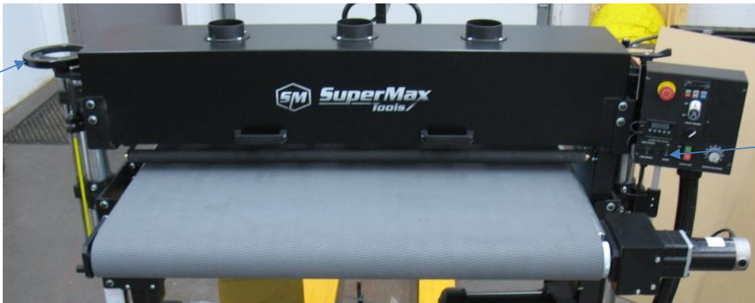
Figure 16: Height Control Adjustments
