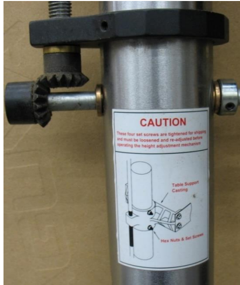
Figure 3: Table Support Set Screws Caution Label
