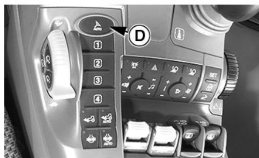
Tractor-Implement Automation™ Button on Tractor Instrument Panel.
