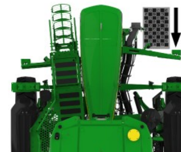
Calibration Board Placement for Front Cameras
