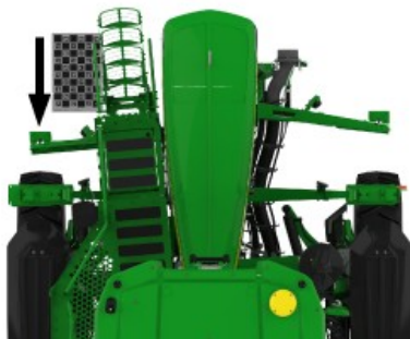
Calibration Board Properly Placed for Front Cameras
