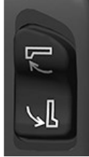
Unloading Auger Switch
