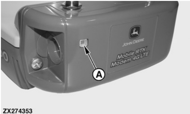
Mobilni RTK modem – Opis LED stanja
