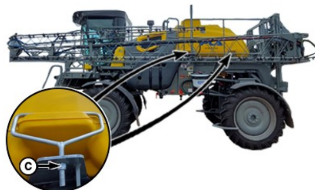
YE1385913—UN—13DEC24 Side Fixing Hardware of the Solution Tank—Machines Equipped with Central Engine
