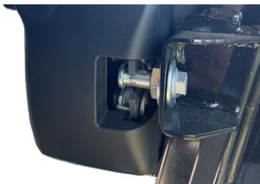
Door Not Fully Locked (Incorrect)
