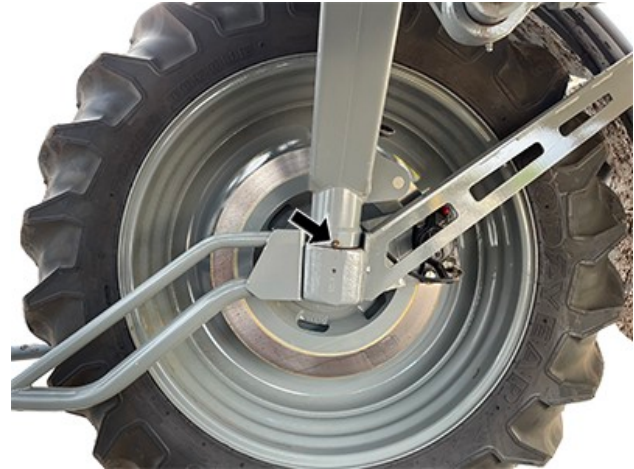
Front Axle Lower Ends—Inner Side (2 greasing points, 1 each side)
