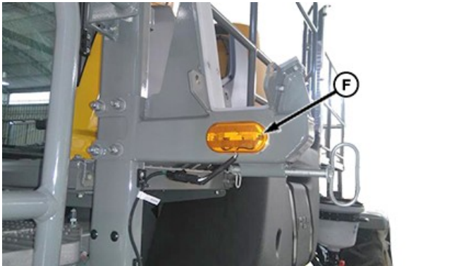
Front Turn-Signal Lights
