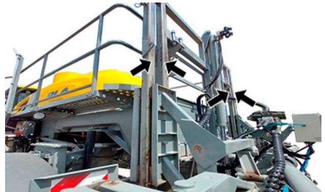
Center Frame Structure (4 greasing points, 2 each side)
