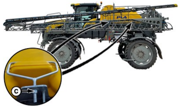
YE001333—UN—02JAN24 Side Fixing Hardware of the Solution Tank—Machines Equipped with Front Engine
