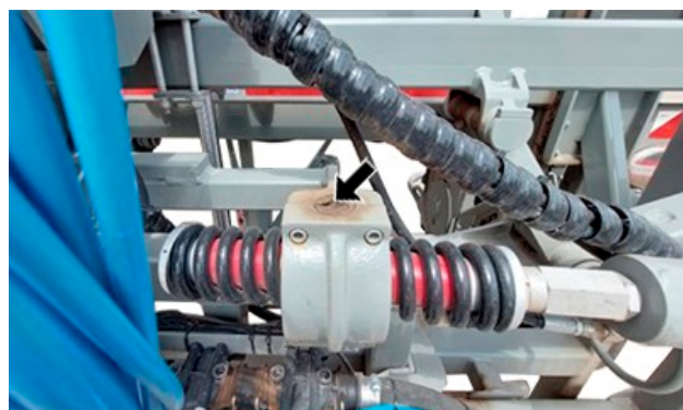
YE000665—UN—30MAR23 Oscillation Lock Cylinder (1 grease fitting)—2900 Self-Propelled Sprayers Only
