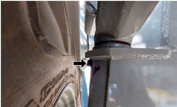
Front Axle Upper Ends—Outer Side (2 greasing points, 1 each side)
