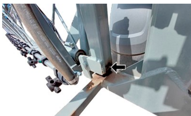
YE000663—UN—30MAR23 Center Frame Lower Hinge Structure (2 greasing points, 1 each side)
