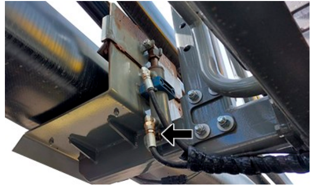
Spray Boom Locking Cylinders (2 greasing points, 1 each side)
