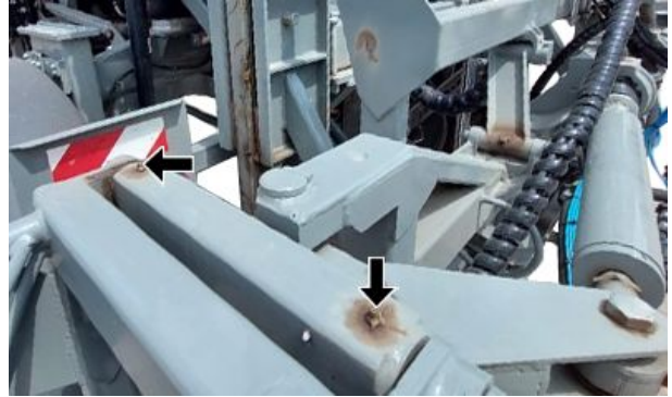
Upper Hinge of the Inner Spray Boom Section (4 greasing points, 2 each side)
