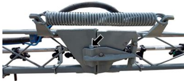
Spray Boom Safety Lock (2 greasing points, 1 each side)
