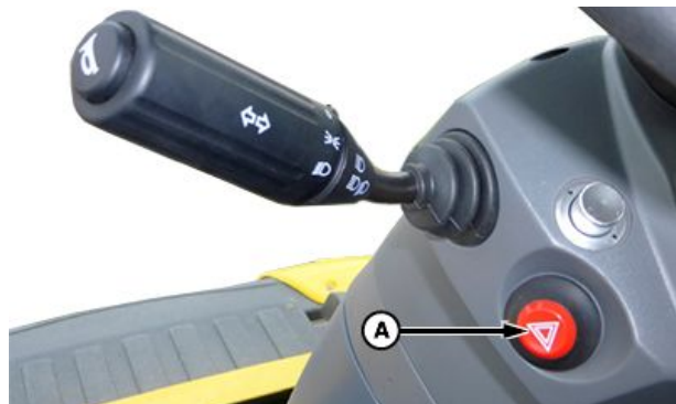
Hazard Warning Light Switch
