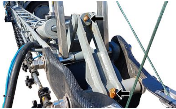
Outer Spray Boom Section Hinge—Outer Side (4 greasing points, 2 each side)
