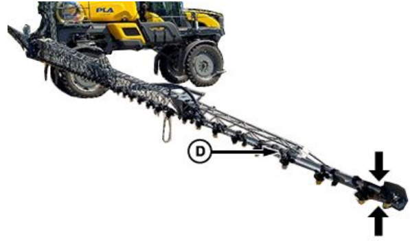
Steel Spray Boom
