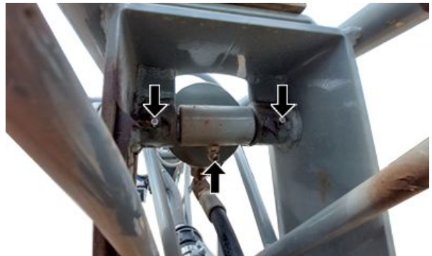
Outer Spray Boom Section Hinge—Cylinder Base Side (6 greasing points, 3 each side)
