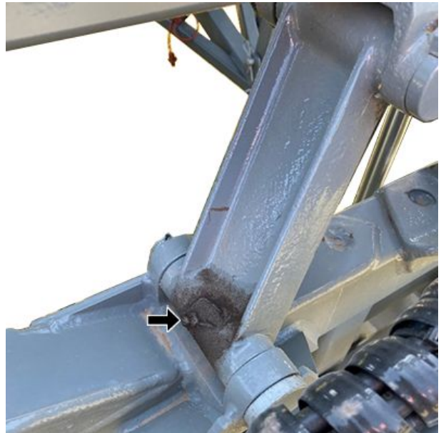
Upper Position Plates of the Oscillation Structure (2 greasing points, 1 each side)—2900 Self-Propelled Sprayers Only
