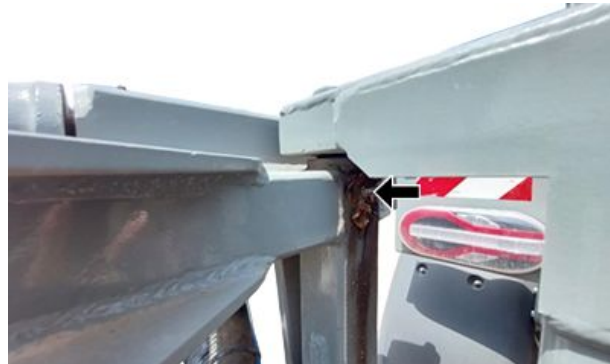
Center Frame Upper Hinge Structure (2 greasing points, 1 each side)
