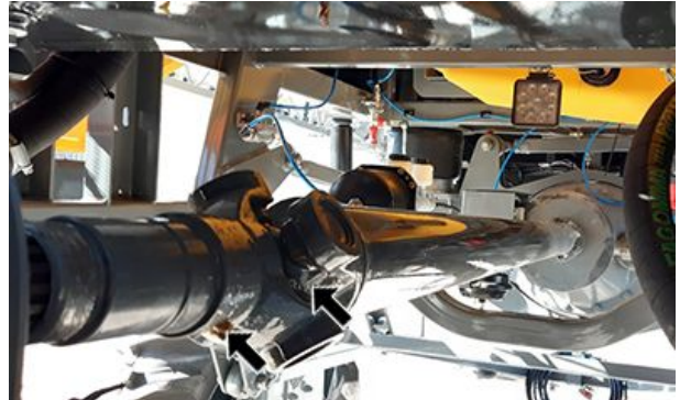
Driveshaft End and Splined Rod (2 greasing points)—Machines Equipped with Front Engine
