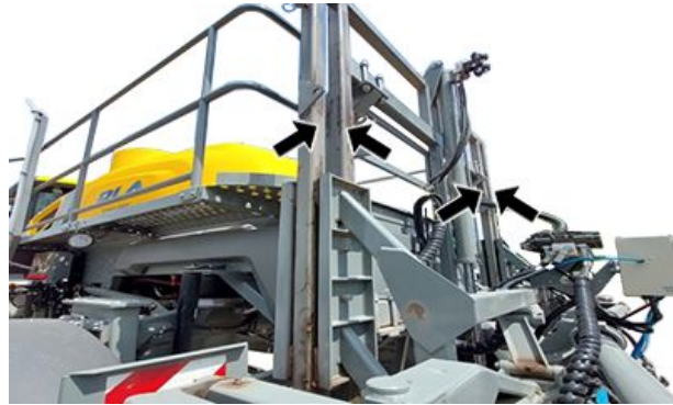
Center Frame Structure (4 greasing points, 2 each side)
