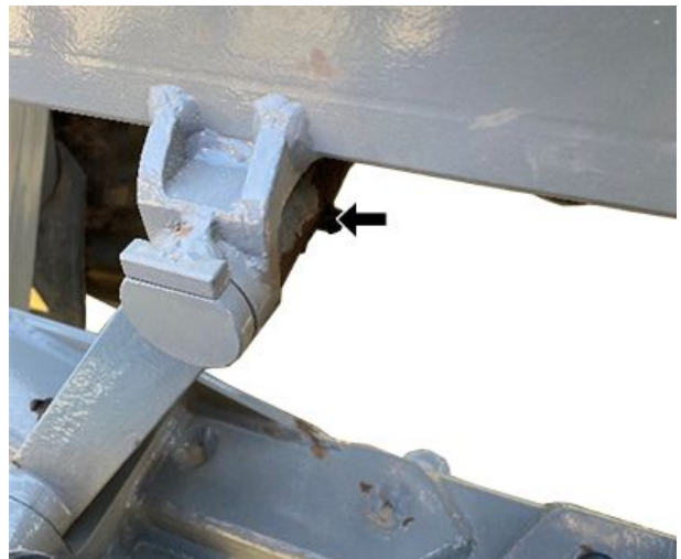
Oscillation Rod—2900 Self-Propelled Sprayer (4 greasing points, 2 each rod)
