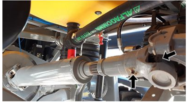
Driveshaft End and Splined Rod (2 greasing points)—Machines Equipped with Central Engine
