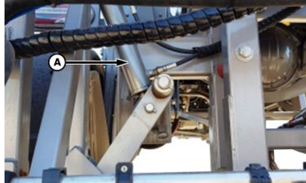
Locking Cylinder—Retracted (unlocked position)
