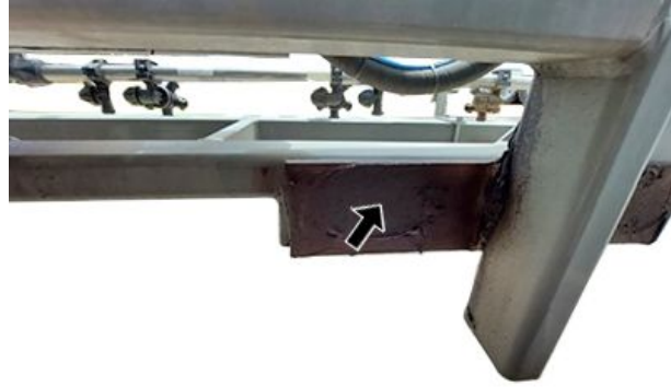
Lower Position Plates of the Oscillation Structure (2 greasing points, 1 each side)
