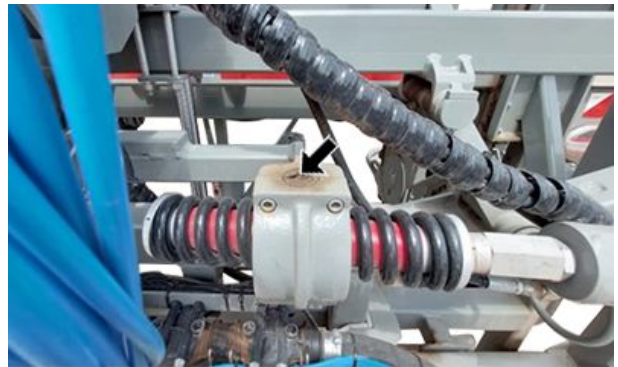
Oscillation Lock Cylinder (1 grease fitting)—2900 Self-Propelled Sprayers Only
