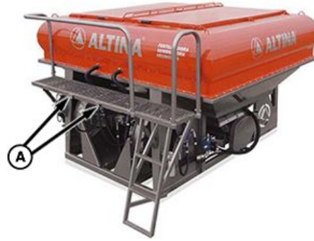
Grease Fittings—Shaft of the Turbines
