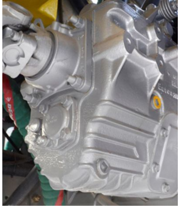
Eaton FS 4205 Transmission-Manual Mechanical Machines
