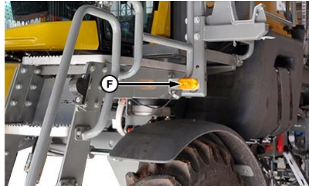
Front Turn-Signal Lights
