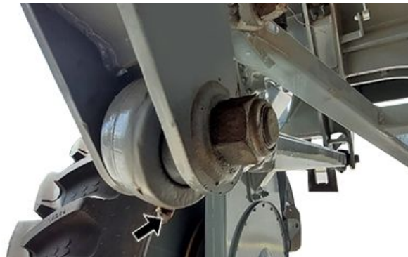
Tensioner Ball Joints (20 greasing points, 2 per tensioner)
