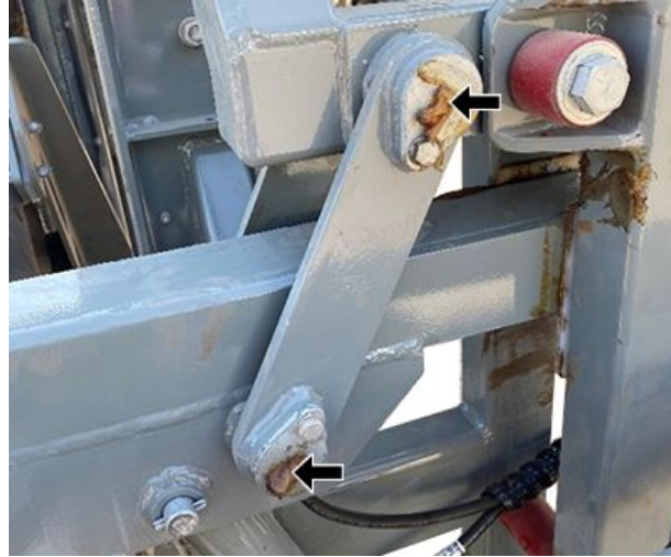
Oscillation Rod—Other Machine Models (4 greasing points, 2 each rod)
