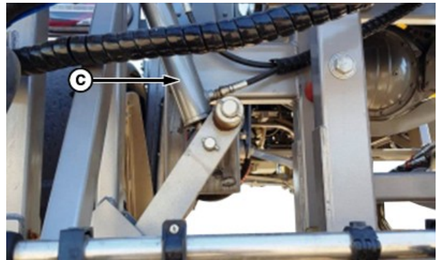
Locking Cylinder—Retracted (unlocked position)
