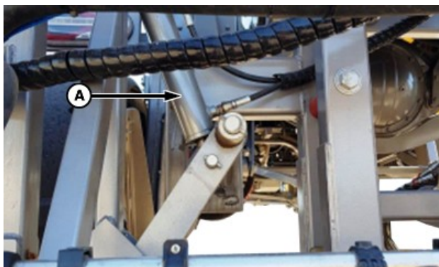
YE000144—UN—22SEP22 Locking Cylinder—Retracted (unlocked position)
