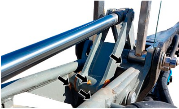
Outer Spray Boom Section Hinge—Inner Side (8 greasing points, 4 each side)
