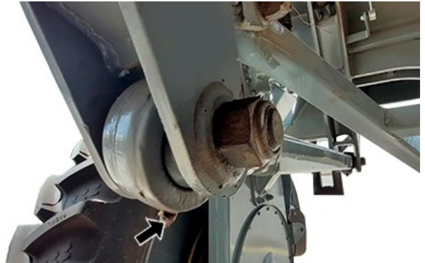
Tensioner Ball Joints (20 greasing points, 2 per tensioner)
