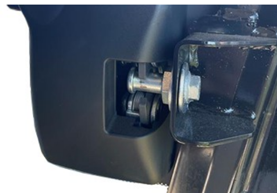
YE1388612—UN—10JAN25 Door Not Fully Locked (Incorrect)
