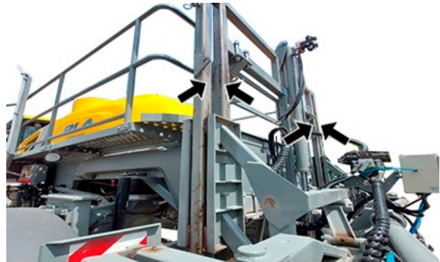
YE000656—UN—30MAR23 Center Frame Structure (4 greasing points, 2 each side)
