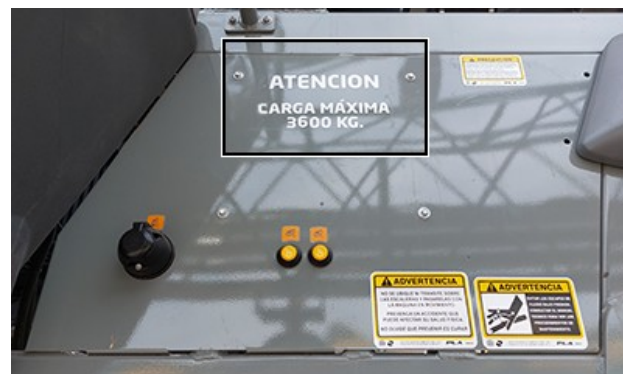
Nutrient Applicator Box Load Capacity (Nutrient Applicator Only)
