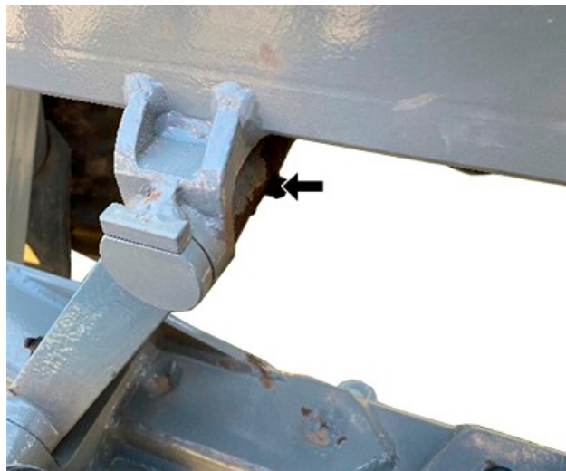
YE000661—UN—30MAR23 Oscillation Rod—2900 Self-Propelled Sprayer (4 greasing points, 2 each rod)
