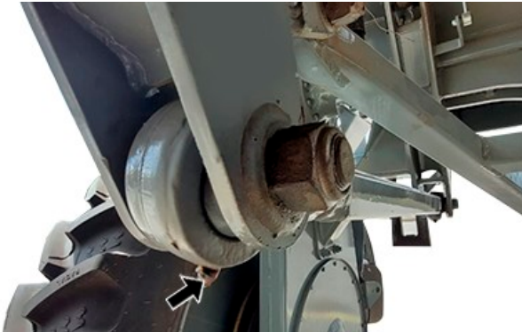
Tensioner Ball Joints (20 greasing points, 2 per tensioner)
