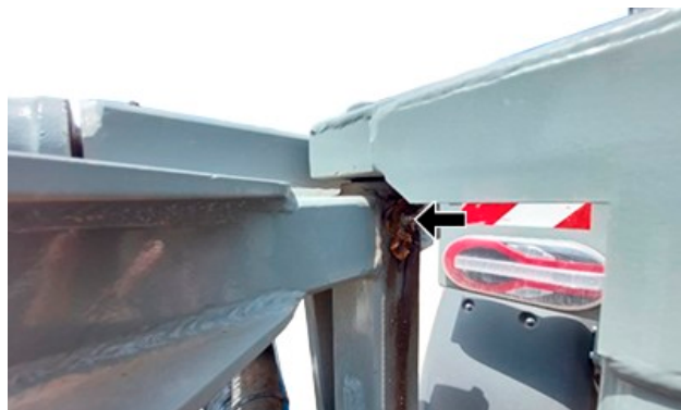
YE000662—UN—30MAR23 Center Frame Upper Hinge Structure (2 greasing points, 1 each side)
