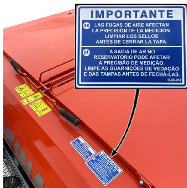
Nutrient Applicator Hopper Pressure (Nutrient Applicator Only)
