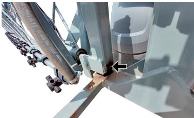
Center Frame Lower Hinge Structure (2 greasing points, 1 each side)
