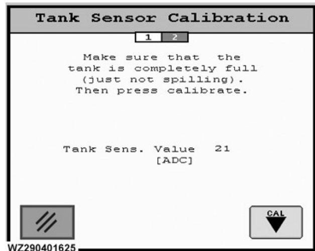
Tank at Overfill Level - Step 2
