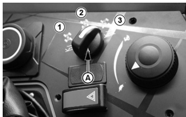
A—Selector Switch 1—Crab Steering 2—Front Wheel 3—4-Wheel Steering
