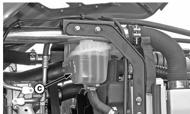
Surge Tank (Deere engine)
