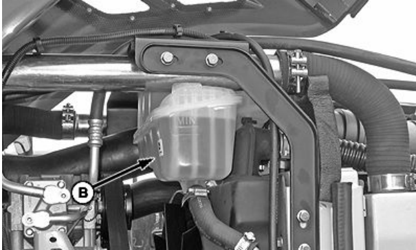
Surge Tank (Deere engine)
