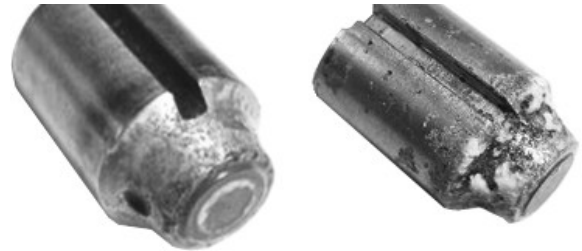
Moderate Corrosion and Pitting
