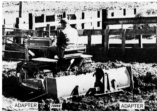
Figure 13—Rear Dozer Adapter Installed
