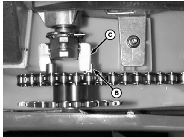
Drives Out Of Alignment
