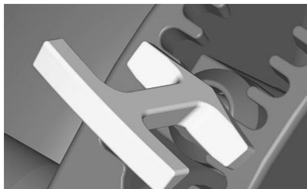
"Walking" The Handle in 6 mm (1/4 in.) Increments
