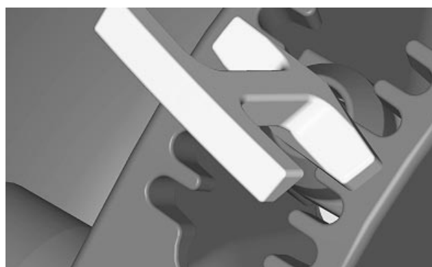
"Walking" The Handle in 6 mm (1/4 in.) Increments
