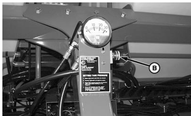
A—Tractor Flow Control Valve B—CCS Flow Control Valve
