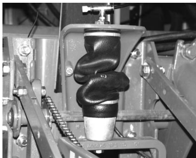
Improperly Rolled Air Spring
