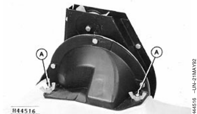
Finger Pick-Up Metering Unit
