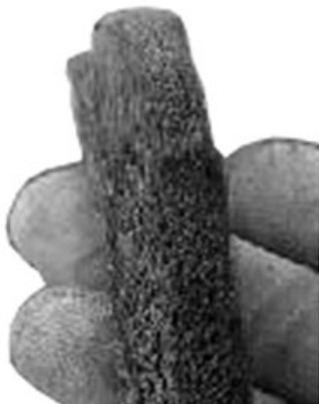
A100144—UN—21MAR18 Desgaste lateral irregular
