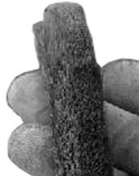
Uneven Side-to-Side Wear
