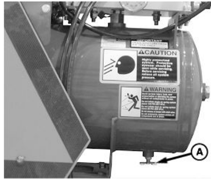
Down Force Air Tank Drain Valve
