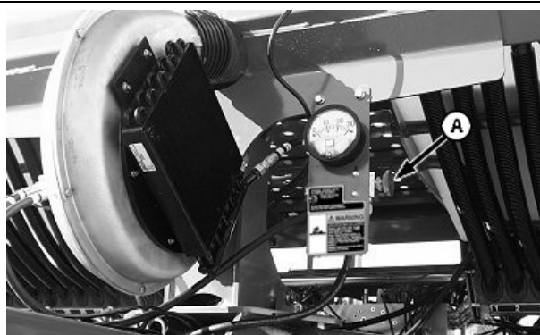
A—Flow Control Valve Handle
