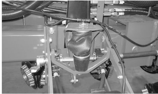
Improperly Rolled Air Spring
