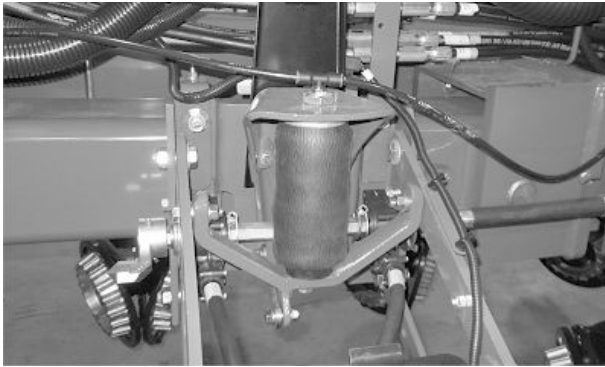
Properly Rolled Air Spring
