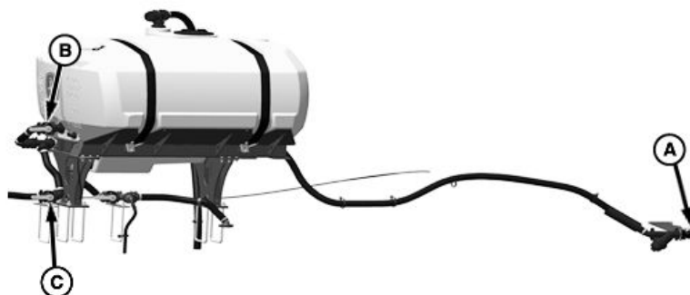
B—Tank Inlet Valve
