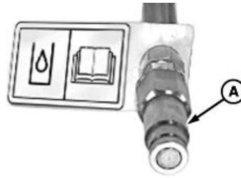
Case Drain Connected First
