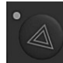
H121091—UN—15MAR17 Hazard Lights (style A)
