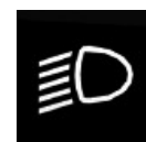
Road Lights Switch
