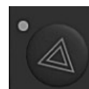
H121091—UN—15MAR17 Hazard Lights (style A)
