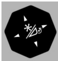
H121181—UN—04APR17 Reel Lift and Fore/Aft Switch (style A)
