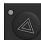
H121091—UN—15MAR17 Havariblinklys (type A)
