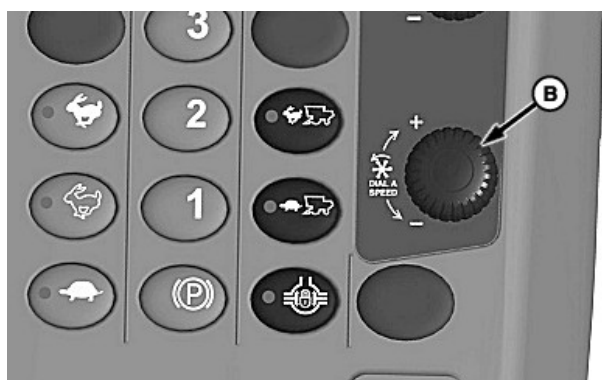
A—Auto Reel/Belt Speed Icon B—Auto Reel/Belt Speed Dial
