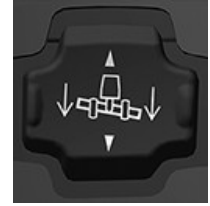
H116348—UN—19DEC16 Header Raise/Lower Switch (style B)
